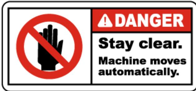
**Danger Stay clear sticker:** Means that the machine moves automatically and will move without warning and cause serious damage to anyone that puts any of there body parts in the area.
